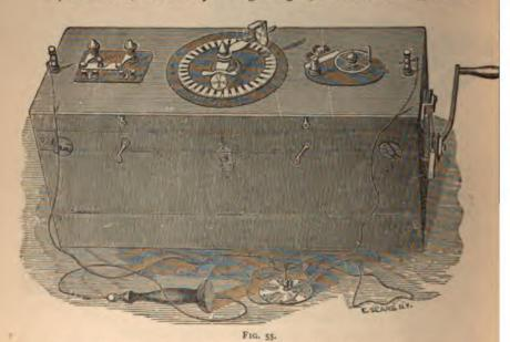
Thirty-six large zinc-carbon cell galvanic battery, with circular switch, reverser, and interrupter, for office or hospital use (Kidder).
